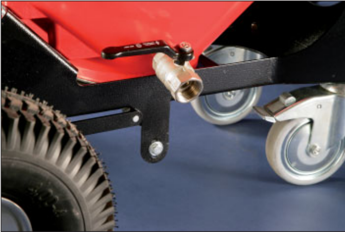
Easy to empty - simply open the tap to drain off the liquid.
