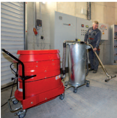
WS 2210 with pre-separator in combined heat and power station
